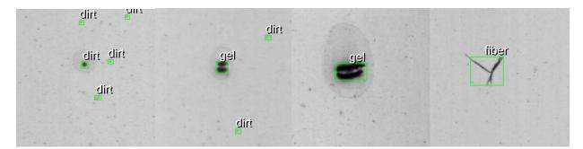
Materials produced in a continous roll or sheet, such as paper, textiles, film, foil, plastics, metals, glass, or coatings, are best inspected by line scan systems. Line scanning offers unlimited pixels in the direction of a web's motion with zero smear even at high speeds, higher dynamic range, greater processing efficiency and much lower price/pixel.
