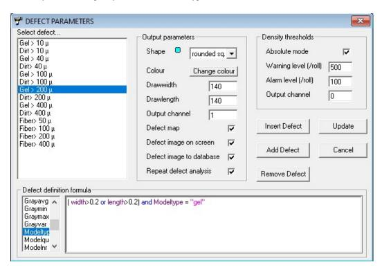
You can create as many modeltypes as you want. Each modeltype consists of a variable number of trained defect models. The classification engine works consistent with a few trained models of each defect type. You don't need a large data set. This leads to a shorter training time and a fast but consequent defect classification.
